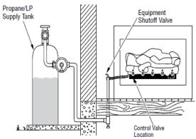
Figure C - External Regulator with Vent Pointing Down
